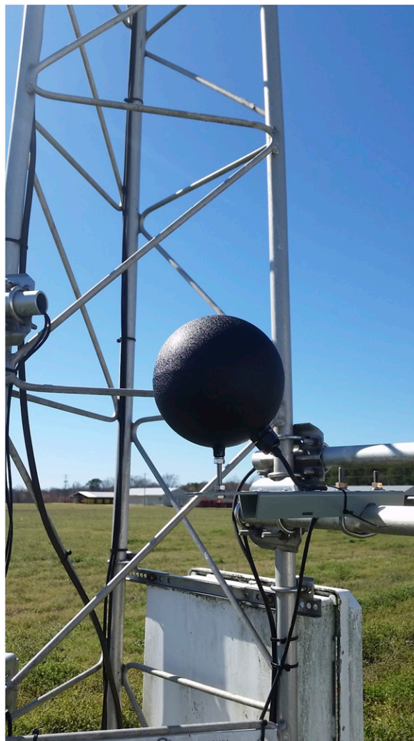
FIG. 1. Black-globe thermometer installed at the North Carolina ECONet Site in Rocky Mount, North Carolina. The image was provided by the NCSCO.
