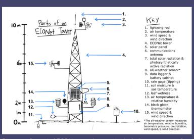
Diagram of a typical ECONet weather station, including power supplies, communications equipment, and environmental sensors.
